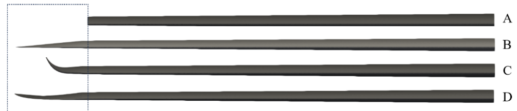
Figure 16. Wingtip configurations: (A) baseline wing, (B) proposed wingtip (flattened winglet), (C) baseline wing with standard UAS-S45 winglet, (D) twist morphing wingtip.
