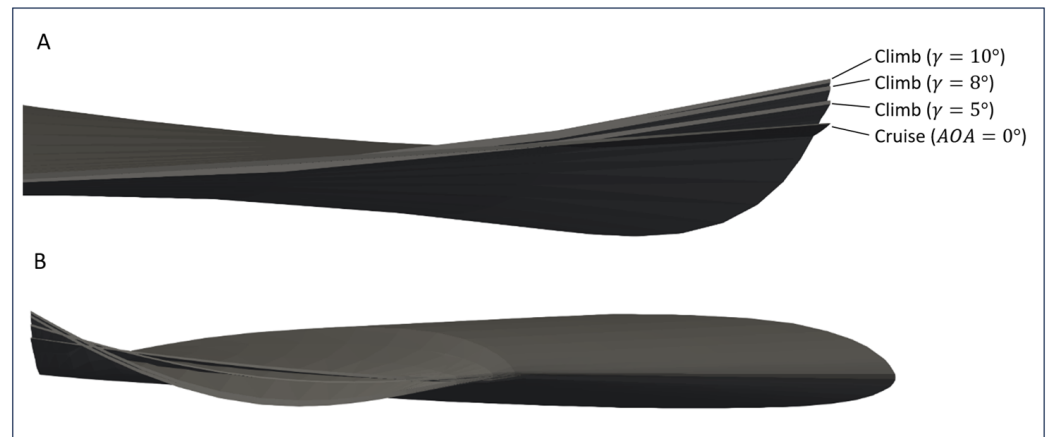
Figure 18. Optimum twist morphing wingtip configuration for four flight conditions: (A) rear view, (B) side view.
