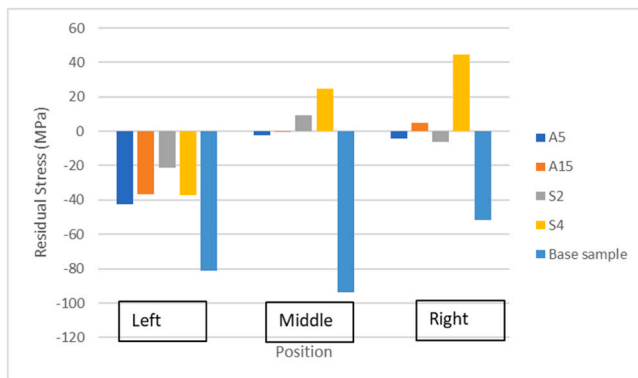
Fig. 14. - Residual Stress measurements on surface.
