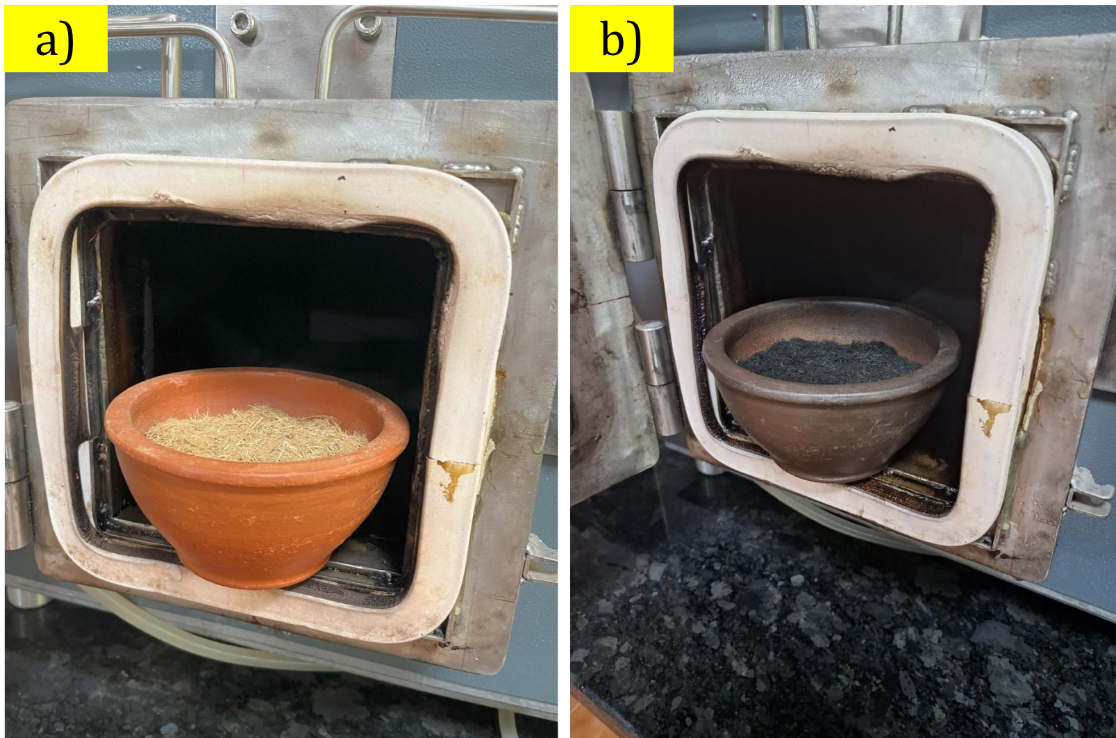
Fig. 5. a) Dried areca nut husk – Before pyrolysis b) AB – After pyrolysis
