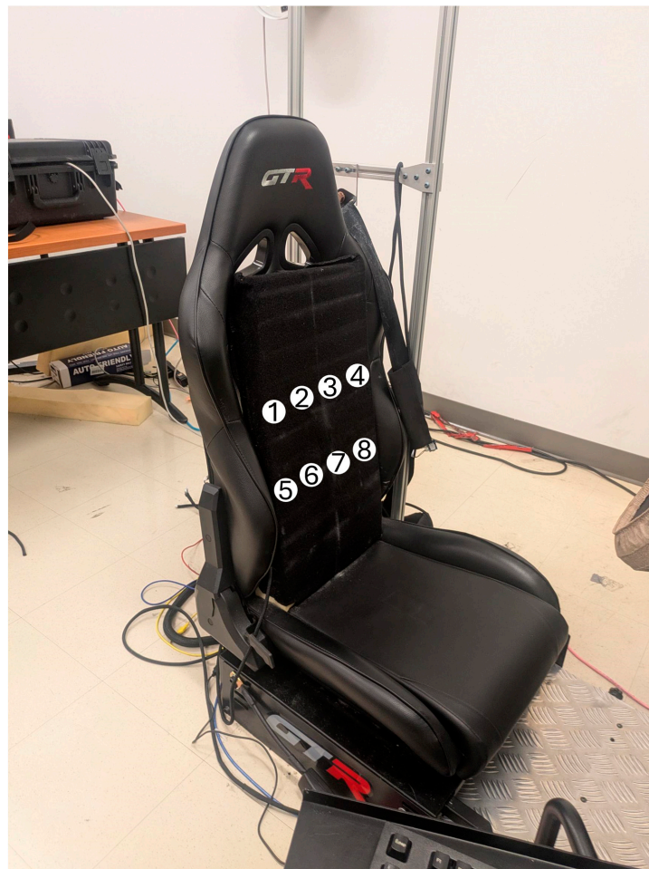
Figure 7. Driving seat and electrode positioning on the seat back. The S105L-BKRD simulator racing seat. A foam covered with loop fabric is used as the seat back. The numbers show approximately where the circular electrodes are attached to the loop fabric during the signal acquisition.
