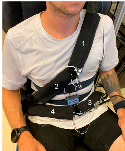
Figure 12. Full electrode integration. Textile inductive electrodes on the seat belt (positions #1, #2, #3, and #4) and the Biopac MP160 respiration strap are shown. Inductive electrodes on the seat back are not visible, hidden by the subject's torso.
