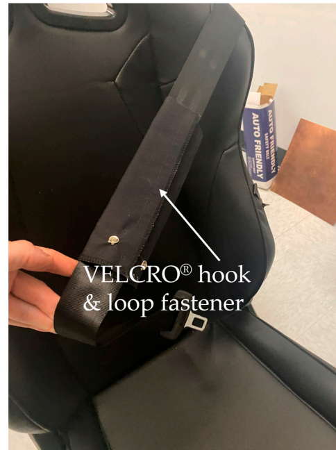
Figure 9. Integration of the electrodes on the seat belt. The electrode is wrapped around the belt with a VELCRO® hook and loop fastener.
