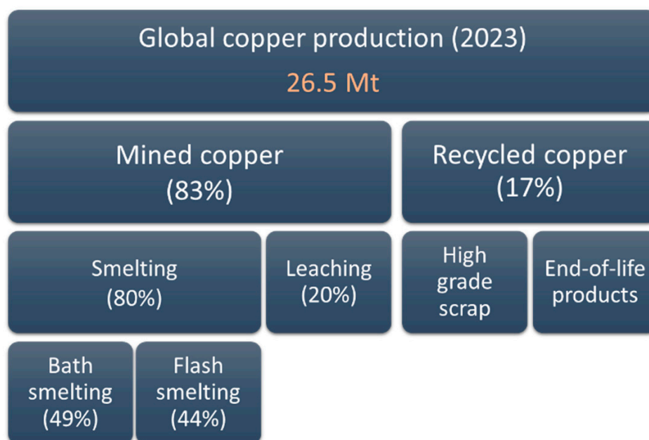
Figure 2. Breakdown of global copper production in 2023, highlighting the share of mined and recycled copper and the distribution of smelting methods (data from [10]).
