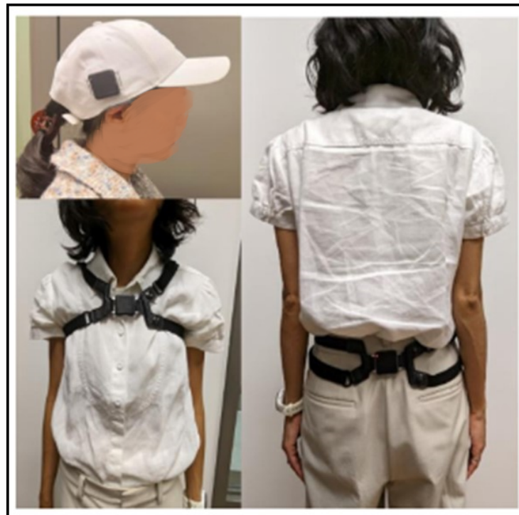
Figure 1. IMU placement locations: head (top left), torso (bottom left), and lower back (right).
