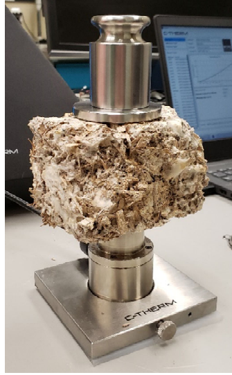
Fig. 1. Thermal conductivity measurement perpendicular to the fibre direction
