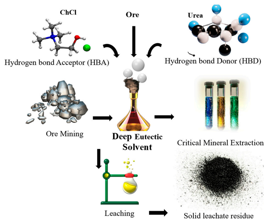
Figure 8. Mineral extraction with DES-based leaching, initiating with choline chloride as the hydrogen bond acceptor and urea as the hydrogen bond donor.
