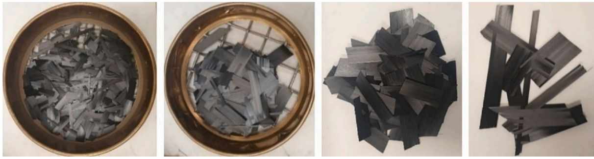
Fig. 7. TET strand aggregates found in a number of different sieves following circular sieving trials.
