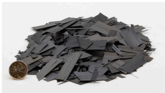
Fig. 1. TET waste from Teijin Carbon America Inc. which has been chopped into strands following polymer impregnation.
