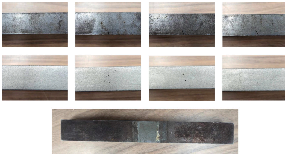
Fig. 4. Different steel samples with defects used during experimental verification.
