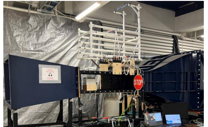
Figure 2. Model wind tunnel experimental setup, showcasing the model scale Vertical Rain Simulation Apparatus, and the sensor enclosure.
