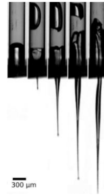
Figure 3. A sequence of liquid jet snapshots captured by an ultrafast camera operating at 60,000 frames per second reveals that flow focusing induces significant acceleration and results in the liquid jet adopting a sharply defined geometrical shape (© 2019. This work is openly licensed via CC BY 4.0) [37].
