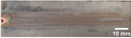
Figure 6. Low power single scan on ETP copper with preheating
