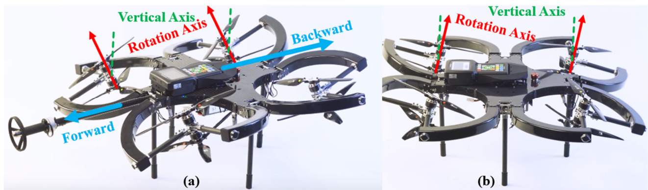
Figure 2. Morphing mechanism of Skygauge: (a) configuration for forward motion, (b) configuration for backward motion [8].
