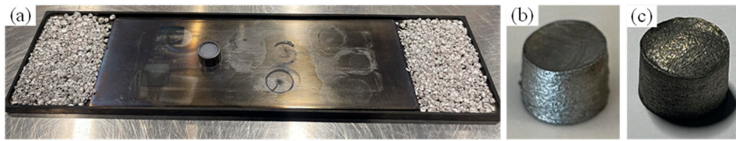
Figure 3. Stainless-steel container with Mg pellets and AlSi10Mg powder before sintering (a) and samples after sintering (b,c): sample #4 (b) and sample #7 (c).
