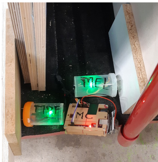
Figure 10. Moisture sensor used for monitoring panel drying conditions.
