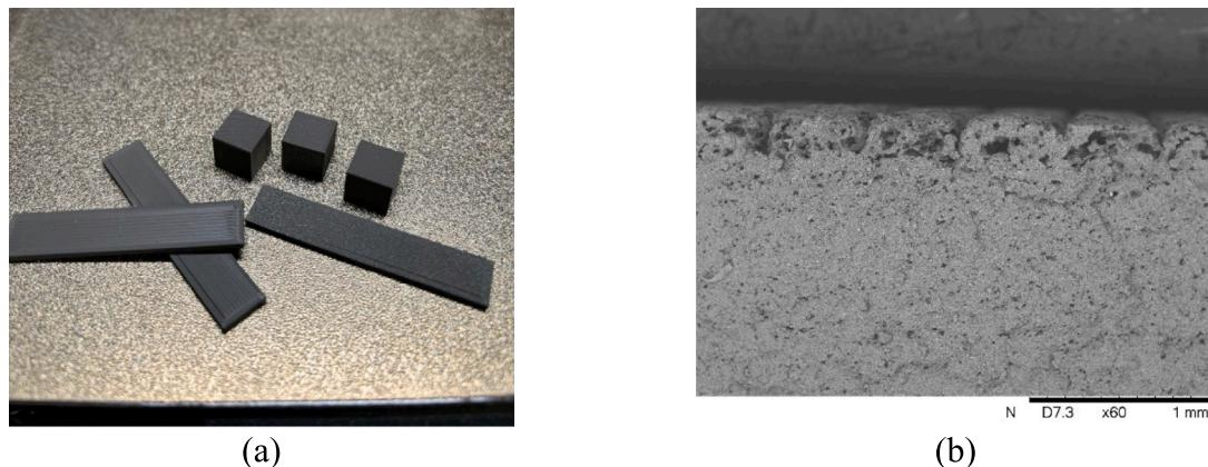
Fig. 14. (a) Optimized 3D-printed parts of Ni-based composite filaments; (b) Printing surface quality for green parts of Ni-based composite filaments. (For interpretation of the references to colour in this figure legend, the reader is referred to the web version of this article.)
