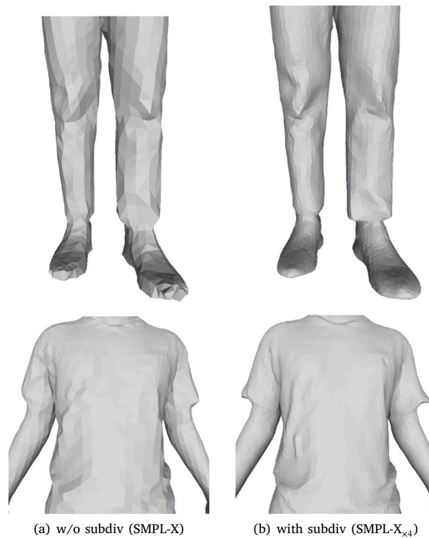
Fig. 12. Comparison without and with mesh subdivision.
