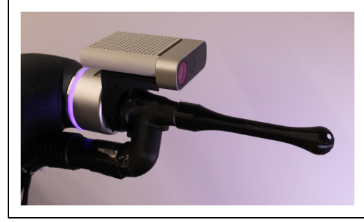
Figure 5. Robot tool with the Azure Kinect camera on the top.
