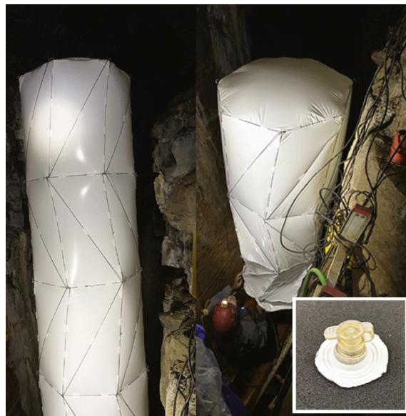
Fig. 15. Envelope performance during a mission in a cave environment: (a) LDPE envelope with a one-way valve assembled in the laboratory, and (b) PU envelope.
