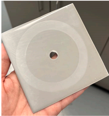
Fig. 7. Surface of the coating after abrasion test, exhibiting minimal wear and no significant damage.
