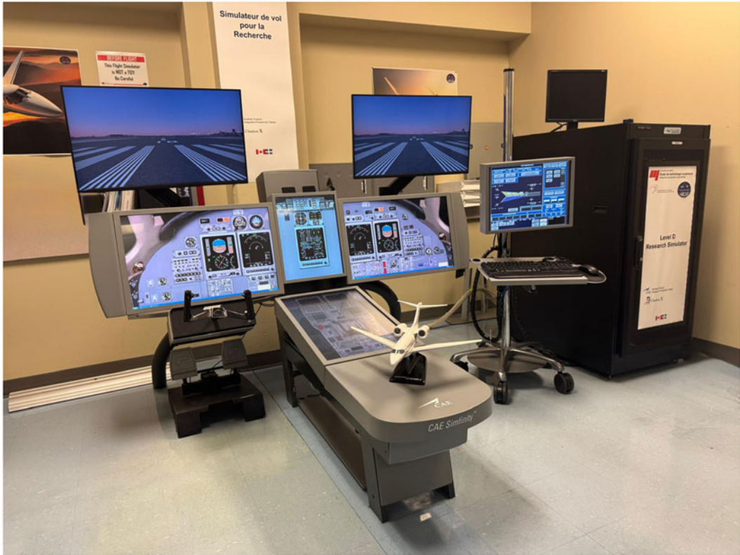
Figure 1. Cessna Citation X research aircraft flight simulator (RAFS) manufactured by CAE Inc.
