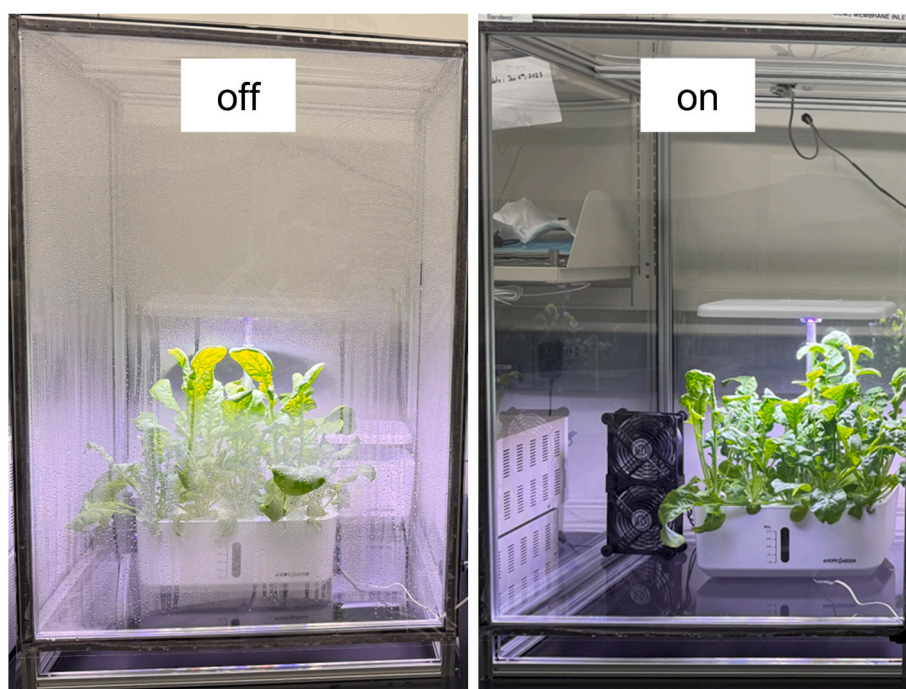
Fig. 1. Humidity control is an important part of creating an ideal plant environment. The image on the left shows a small plant chamber in our laboratory, operating without any humidity control, and high humidity can clearly be seen with condensation of the clear enclosure. The image on the right shows the same system with proper dehumidification.
