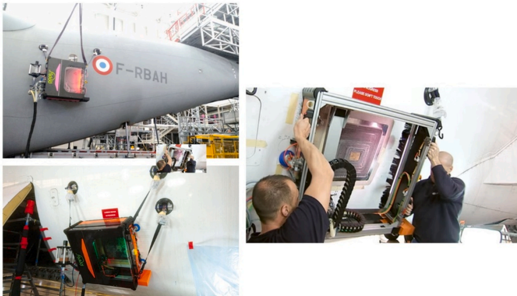
Fig. 13. In-situ composite repair of aircraft components using a portable AWJM system [209].
