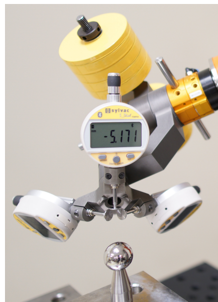
Figure 2. TriCal system during automated reference sphere probing.
